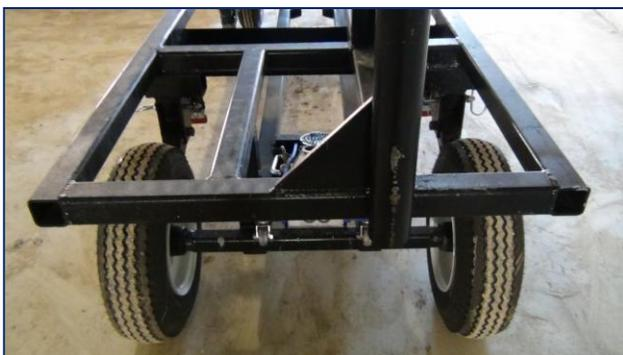
Figure 4. Heavy duty frame and tires.
